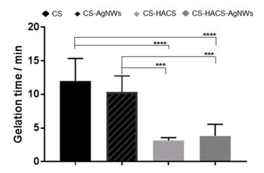
**Figure S3.** Physical characterisation of the hydrogels: CS (black), CS-HACS-AgNWs (black background with dark grey lines), CS-HACS (light grey) and CS-HACS-AgNWs (dark grey). Gelation time calculated by the inverted tube method. Data are reported as mean  $\pm$  SD (n = 9). One-way ANOVA returned p < 0.0001. Post-hoc Tukey's comparison test results are shown in the graph: \*\*\*\* indicates p < 0.0001 and \*\* indicates p < 0.001.
