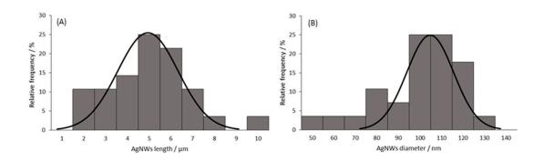
Figure S1. AgNWs size distribution obtained by SEM image analysis. (A) Length (mean  $5.03 \pm 1.85 \, \mu m$ ; n = 28) and (B) diameter (mean  $99.45 \pm 20.20 \, nm$ , n = 28). Shapiro-Wilk normality test returned p > 0.05 for both length and diameter.
