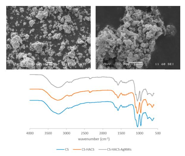
Figure S2. SEM images of HACS (top) and FTIR spectra of the three hydrogels (bottom).
