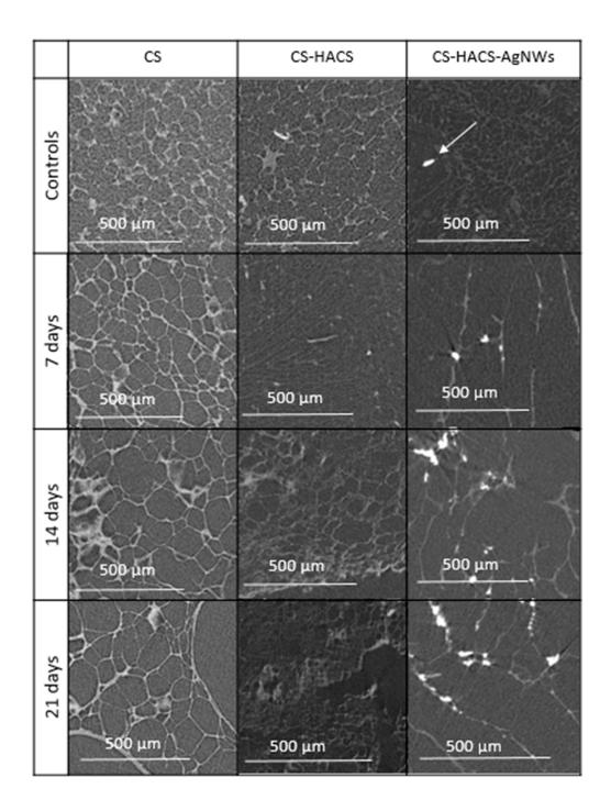
**Figure S6.** MicroCT images of CS, CS-HACS and CS-HACS-AgNWs hydrogels incubated in SBF for 7, 14 and 21 days. The arrow indicates an area of mineralized tissue characterized by a higher X-ray absorption than the surrounding hydrogel.
