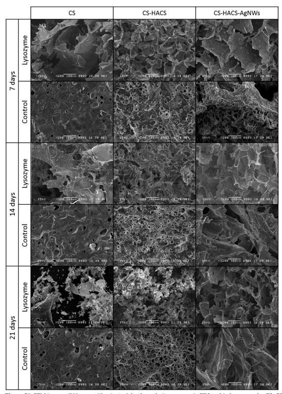
**Figure S5**. SEM images (200× magnification) of the degradation process in PBS and in lysozyme for CS, CS-HACS and CS-HACS-AgNWs gels at 7, 14 and 21 days.
