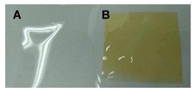
Figure S1. Photographic images of non-crosslinked (A) and crosslinked (B) solvent cast (SC) films.
