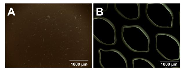
**Figure S2**. Optical microscopy images of non-crosslinked solvent cast (SC) film (A) and bi-layered solvent cast/3D printed (SC/3D) carrier (B).
