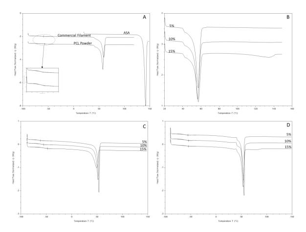
**Figure S3.** DSC thermograms of **A**) Raw materials. **B**) ASA-PCL powder mixtures (first heating cycle). **C**) ASA-PCL powder mixtures (second heating cycle). **D**) HME fabricated filaments.
