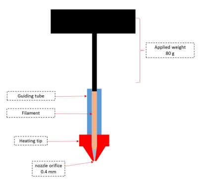
**Figure S2.** Illustration for the method adapted for measuring the melt flow index (MFI) for different materials.
