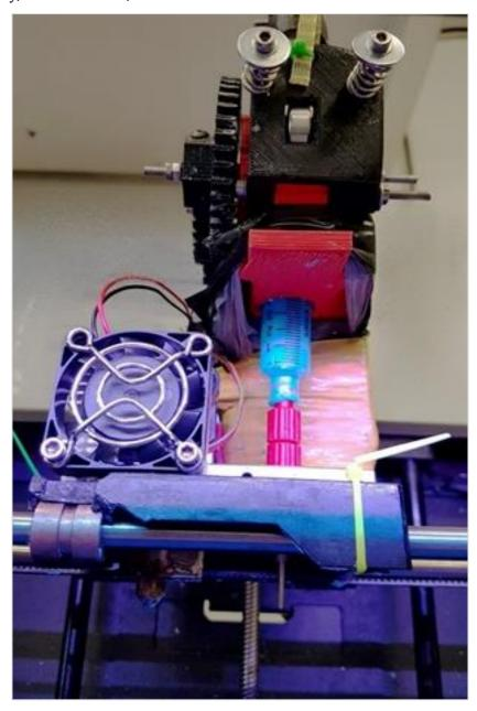
**Figure S1.** Modification of dual FDM 3D printer to accommodate a liquid/semisolids dispenser (right) in combination with FDM 3D printer head (left).
