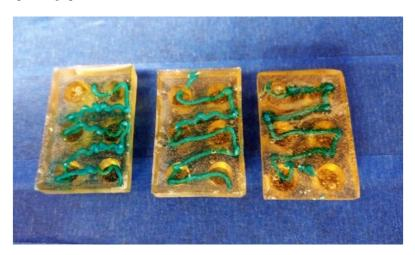
**Figure S3.** Soft dosage forms with paracetamol inside (blue line) fabricated via one-step e-3DP with printing speed 55.0mm/min.
