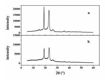
Figure 1. XRD diagram of the HK SD prepared (a) one week prior and (b) 16 months prior.
