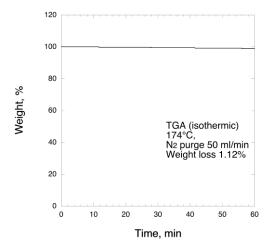
Figure 1. Thermogravimetric analysis (TGA) profile of NIF maintained at 174 °C for 1 h.
