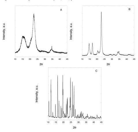
Figure 2. XRD profiles of MCC (A), CLAD (B) and NIF (C).
