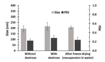
Figure S3: Mean dimensions and PDI of NHs before and after the addition of dextrose ( $C_f = 1\% \text{ w/V}$ ), and after freeze-drying and re-suspension in water
