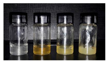
**Figure S5.** Image of the prepared HPMC/CS mixed hydrogels in 200 mM acetate buffer pH 4.5. From left to right: 5.5% HPMC (control); 5.5% HPMC/1%CS; 5.5% HPMC/1%CS NPs 12:1; 5.5% HPMC/1%CS NPs 6:1.
