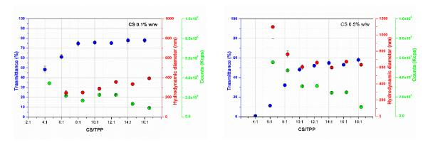
**Figure S4.** Hydrodynamic diameter (nm), counts (Kcps) and transmittance (%) of nanoparticles at different CS concentrations (0.1%, 0.5% and 1% w/w) and different CS/TPP ratios prepared in acetate buffer pH 5.5.
