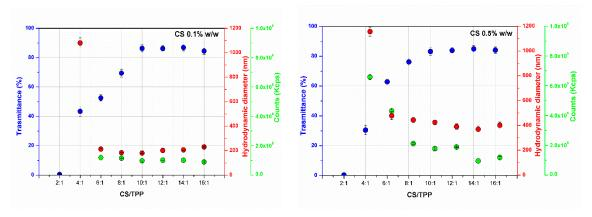
**Figure S3.** Hydrodynamic diameter (nm), counts (Kcps) and transmittance (%) of nanoparticles at different CS concentrations (0.1%, 0.5% and 1%; w/w) and different CS/TPP ratio prepared in acetate buffer pH 5.
