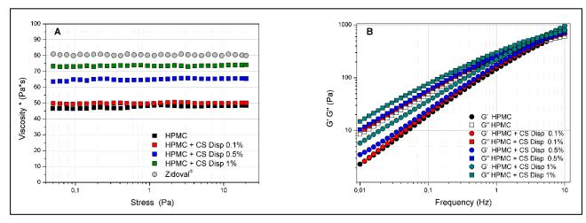
**Figure S6.** Stress sweep **(A)** and frequency sweep **(B)** results obtained from HPMC/CS mixed hydrogels at 37 °C. CS was dispersed into HPMC as a free polymer.
