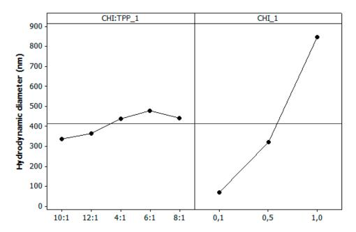
**Figure S1.** "Main effect" plot relative to the factors (CS % and CS/TPP ratio) influencing the size of nanoparticles.
