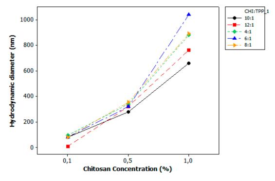
**Figure S2.** "Interactions plot" between the factors (CS % and CS/TPP ratio) influencing the size of nanoparticles.
