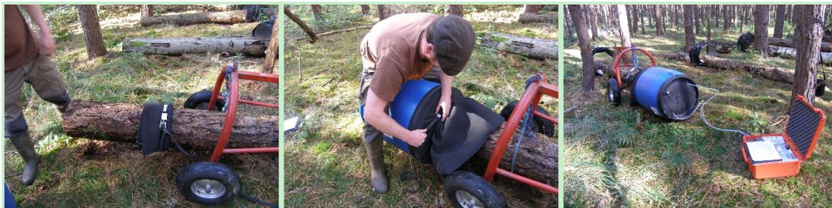
**Figure 1.** Closed chamber system used for CO<sub>2</sub> emission measurements under field conditions.
