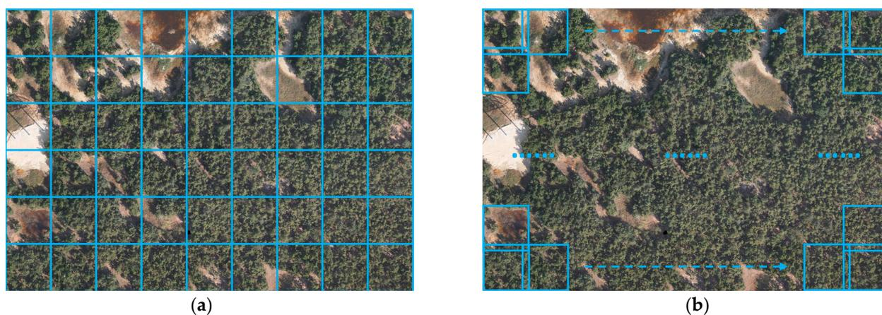
**Figure 2.** Schematic diagram of image cropping with (a) regular grid and (b) overlapping region, respectively.
