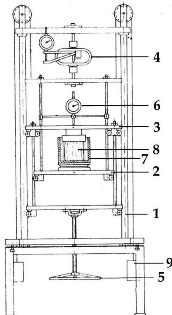
**Figure 3.** A scheme depicting the equipment used for the measurement of swelling pressure; 1—a stand, 2 and 3—slidable frames, 4—dynamometer, 5—adjusting screw, 6—dial micrometre, 7—container filled with water, 8—sample, and 9—weights.
