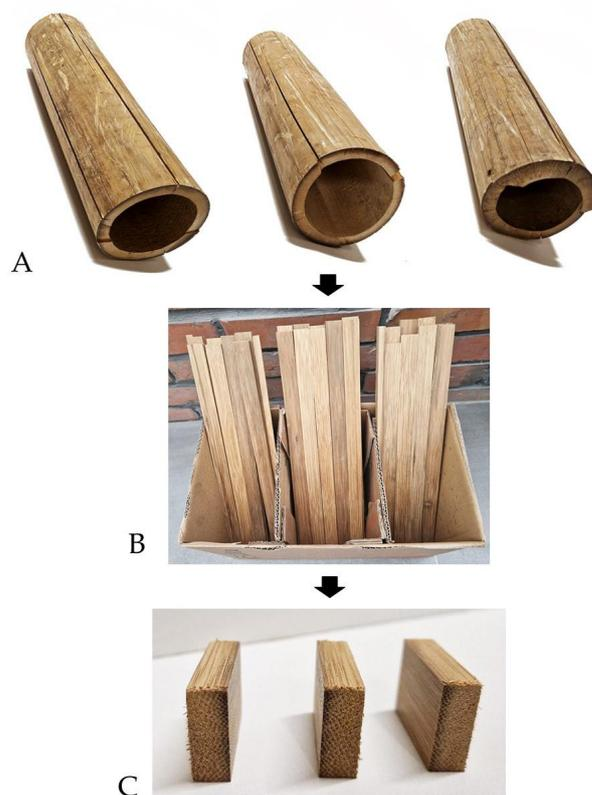
**Figure 1.** A scheme showing research material: (A) three bamboo internodes, (B) slats cut from bamboo internodes, and (C) final samples used in the research.
