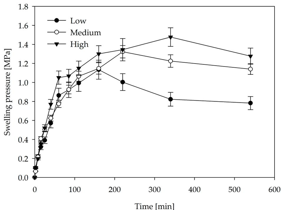
**Figure 5.** Swelling pressure graph for three different density groups of bamboo blocks: low, medium, and high. Measurements were conducted in the tangential direction; error bars represent the standard deviation.
