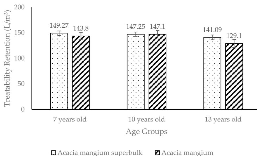
**Figure 11.** Treatability retention of *Acacia mangium* superbulk and *Acacia mangium* [9].
