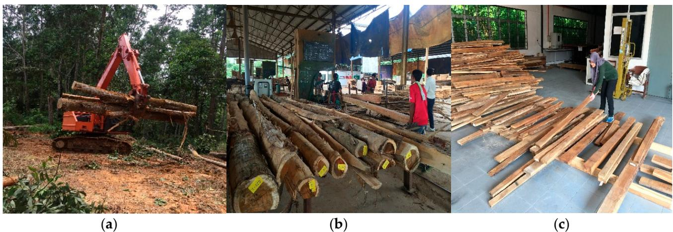
**Figure 1.** *Acacia mangium* superbulk timber collection: (a) the timber logs were transferred out from the plantation site; (b) the timber logs were cut into the plank size; (c) the timber planks were arranged and stacked according to tree numbers for drying.
