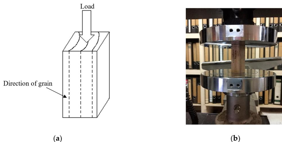
Figure 4. (a) The compression parallel to the grain test [13]; (b) the compression parallel to the grain test at the laboratory.
