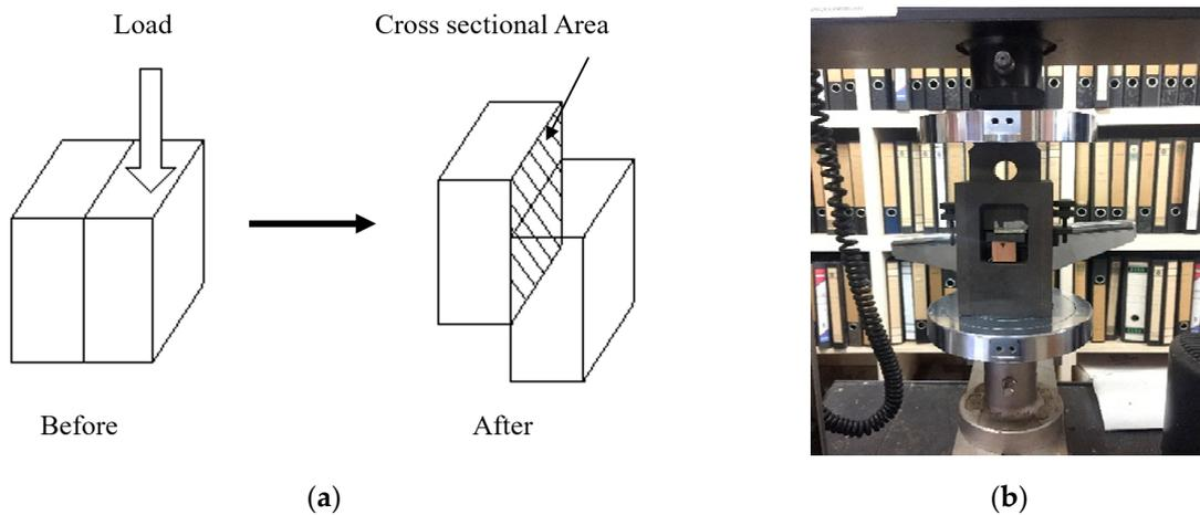
**Figure 5.** (a) The shear parallel to the grain test [13]; (b) the shear parallel to the grain test at the laboratory.
