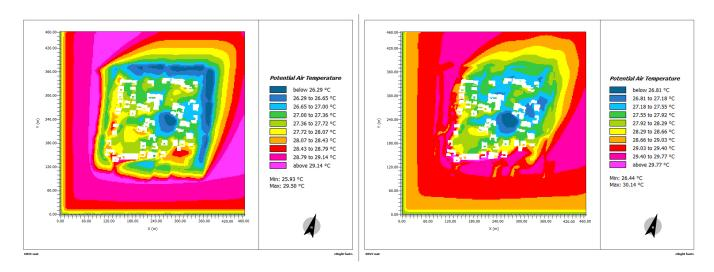
**Figure 7.** Air temperature distribution at 15:00 on 21 June 2021 (with water bodies on the left and without water bodies on the right).
