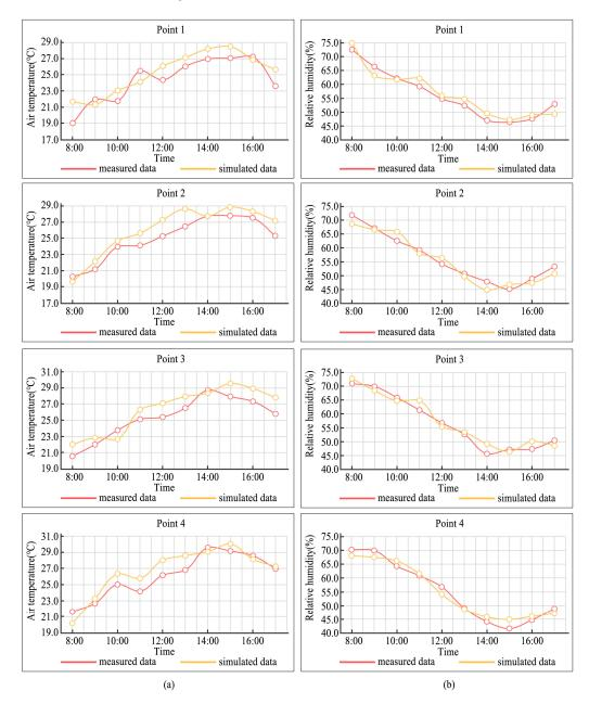
**Figure 5.** Comparison of the simulated and measured data at 1.5 m above the ground at four measuring points used to verify the effectiveness of the ENVI-met software: (**a**) air temperature and (**b**) relative humidity.
