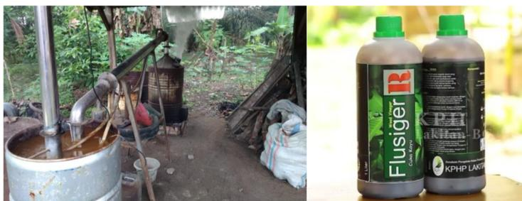
**Figure 9.** Location and apparatus utilized for producing liquid smoke, including the modified drum furnace and condenser (left), and liquid smoke products that are for commercialization (right).
