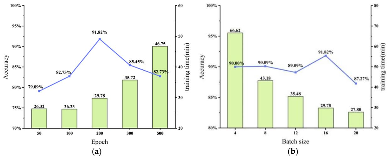
**Figure 7.** Accuracy of different (a) epochs (200) and (b) batch sizes (16).
