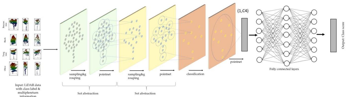
**Figure 3.** Workflow of PointNet++ used in the experiment.
