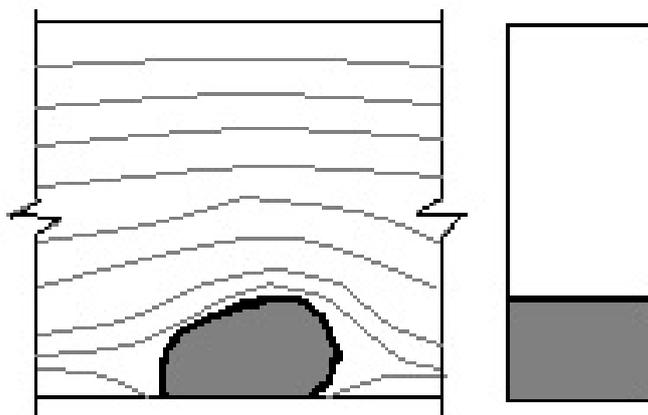
Figure 10. Cross-sectional reduction due to edge knots.
