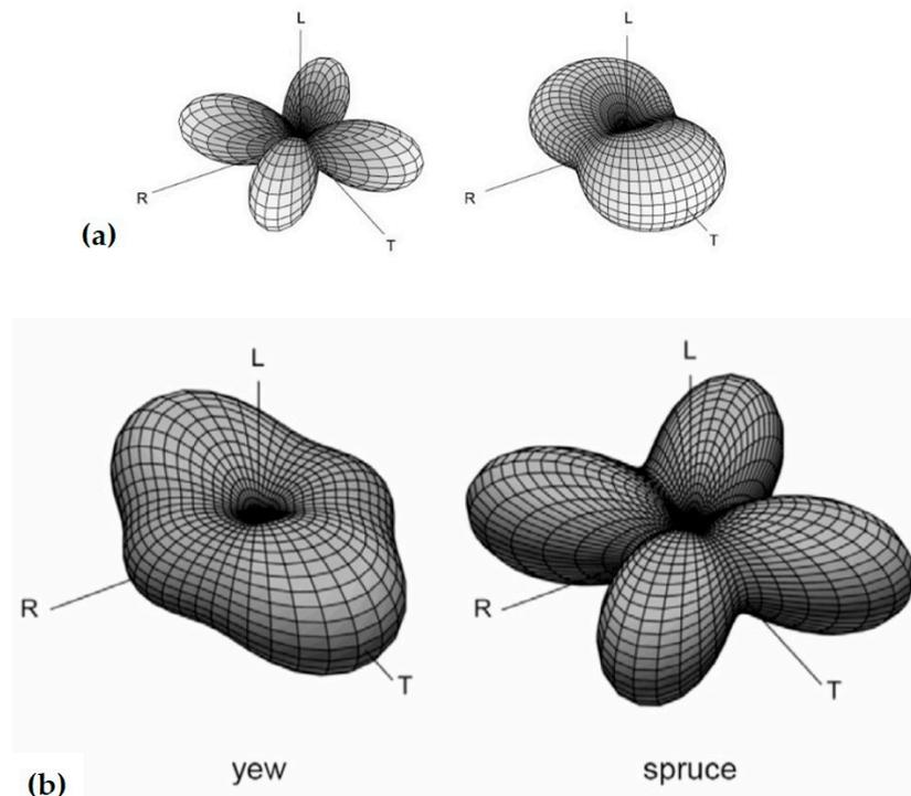
**Figure 7.** Deformation body of wood. (a) Spruce and beech wood in normal climate according to ([33], source [15], (courtesy of Carl Hanser Verlag GmbH & Co. KG, Munich); (b) Yew and spruce under tensile load [17] (Courtesy of D. Keunecke).
