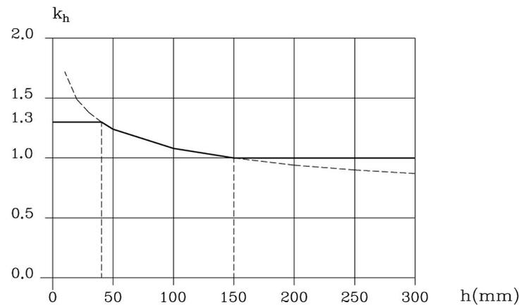
**Figure 27.** Depth factor  $k_h$ , in sawn timber. Design value in a continuous line and Equation (4) in a dotted line (from Arriaga et al. [179]).
