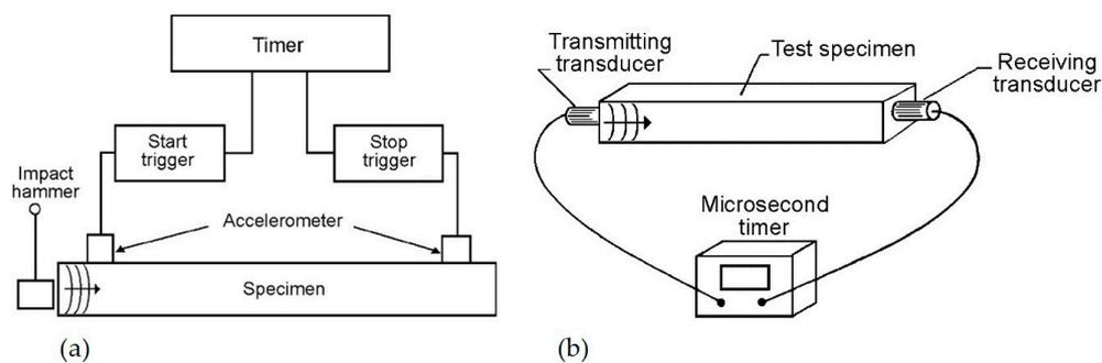
**Figure 17.** TOF acoustic measurement system used to measure longitudinal wave velocity in a wood member through (a) mechanical impact, and (b) ultrasonic waves (source: [87], courtesy of the USDA Forest Service, Forest Product Laboratory, Madison, WI, USA).
