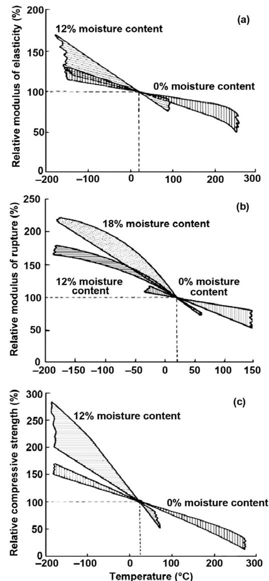
**Figure 25.** Effects of temperature on wood properties at two moisture content levels relative to value at 20 °C for clear, defect-free wood. (a) Modulus of elasticity parallel to grain; (b) modulus of rupture in bending; (c) compressive strength parallel to grain [60] (courtesy of the USDA Forest Service, Forest Product Laboratory, Madison, WI, USA).
