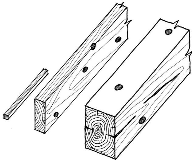
**Figure 9.** Left to right: Small-size clear specimen, Structural-size medium and large cross-section (Credit: GICM-UPM).
