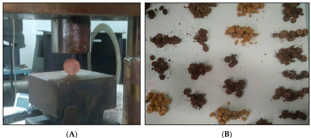
**Figure 2.** (A) Mechanical durability test of 100% bark pellet and (B) destroyed pellet samples after the completion of the testing process.
