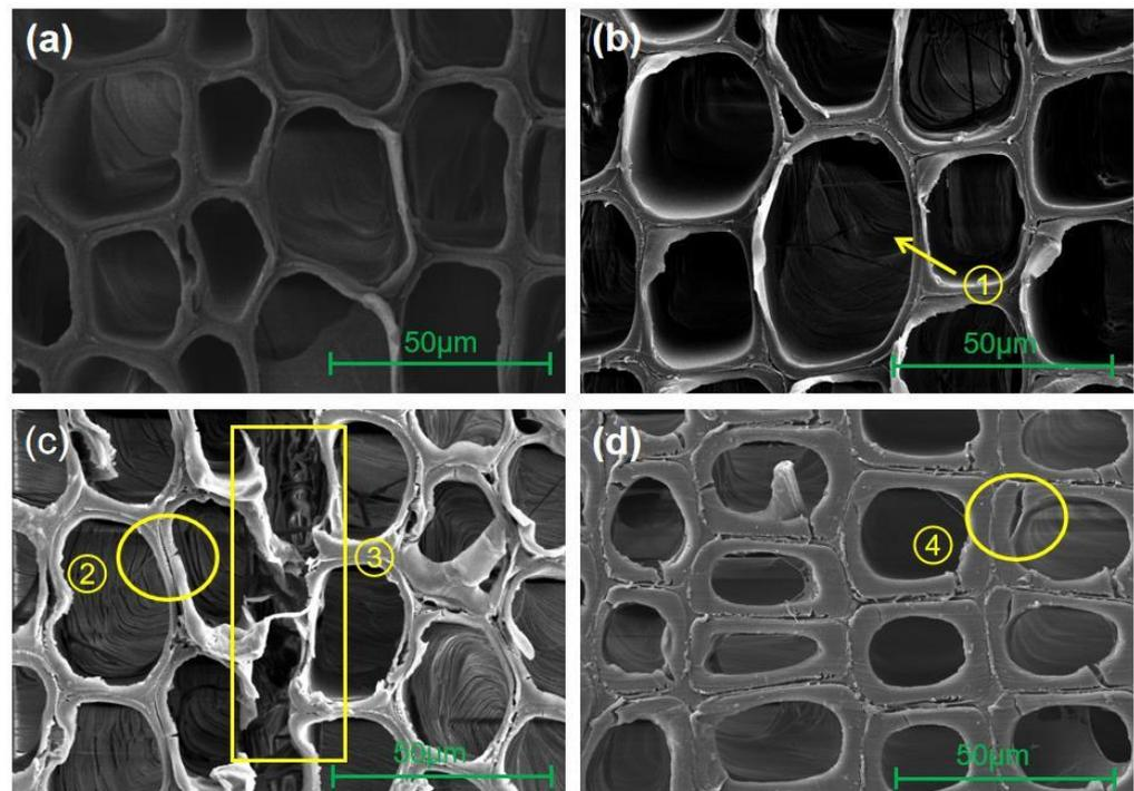
**Figure 3.** SEM images of cross-sections at different incubation times. (a) the control sample; (b) 4-week inoculated sample with *T. versicolor*, ① hyphae were visible in tracheid lumina; (c) 8-week inoculated sample of *T. versicolor*, ② tiny cracks appeared in the tracheid cell walls, ③ ray parenchyma cells were strongly degraded; (d) 12-week inoculated sample of *T. versicolor*, ④ many visible cracks in tracheid cell walls.
