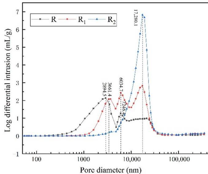
**Figure 4.** Log differential intrusion versus pore diameter of control and inoculated samples.
