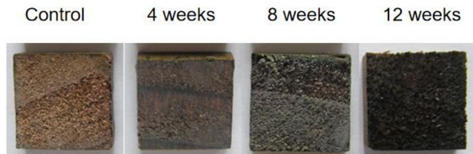
**Figure 1.** Preservative penetration at the cross-section of specimens.
