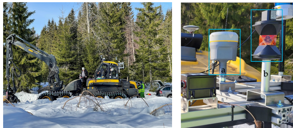
Figure 2. The Ponsse Ergo harvester and the equipment installation on its roof: the Trimble R12 (a); the prism (b).
