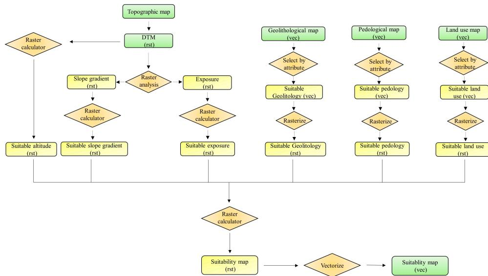
**Figure 3.** Flowchart of GIS-based processing for suitability map building. Between brackets, rst and vec indicate raster and vector file types, respectively.
