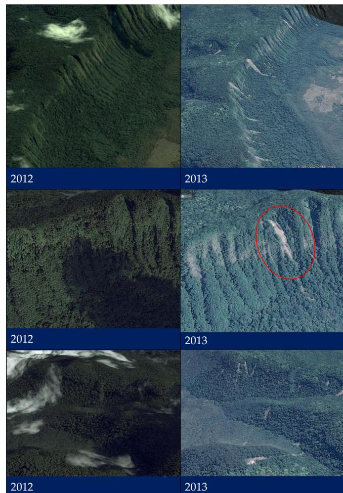
**Figure 3.** Images assembled from Google Earth, displaying significant historic disturbance events at Main Range National park between 2012–2013. The landslips post the 2012 flooding can be identified as the exposed ground or cleared hill face (for example, see red circle).
