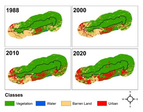
Figure 3. Supervised classification (maximum likelihood) from 1988 to 2020.
