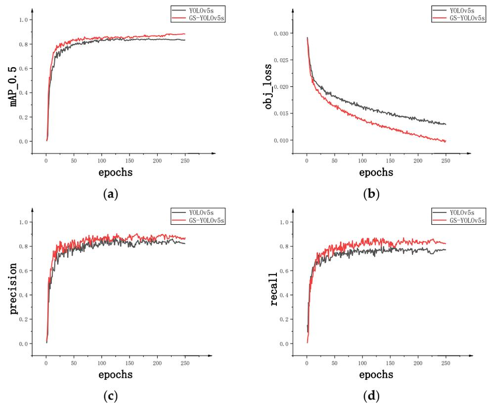
**Figure 10.** (a) Comparison of the mean average precision between GS-YOLOv5s and YOLOv5s. (b) Comparison of the regression Loss function between GS-YOLOv5s and YOLOv5s. (c) Comparison of the precision between GS-YOLOv5s and YOLOv5s. (d) Comparison of the recall between GS-YOLOv5s and YOLOv5s.
