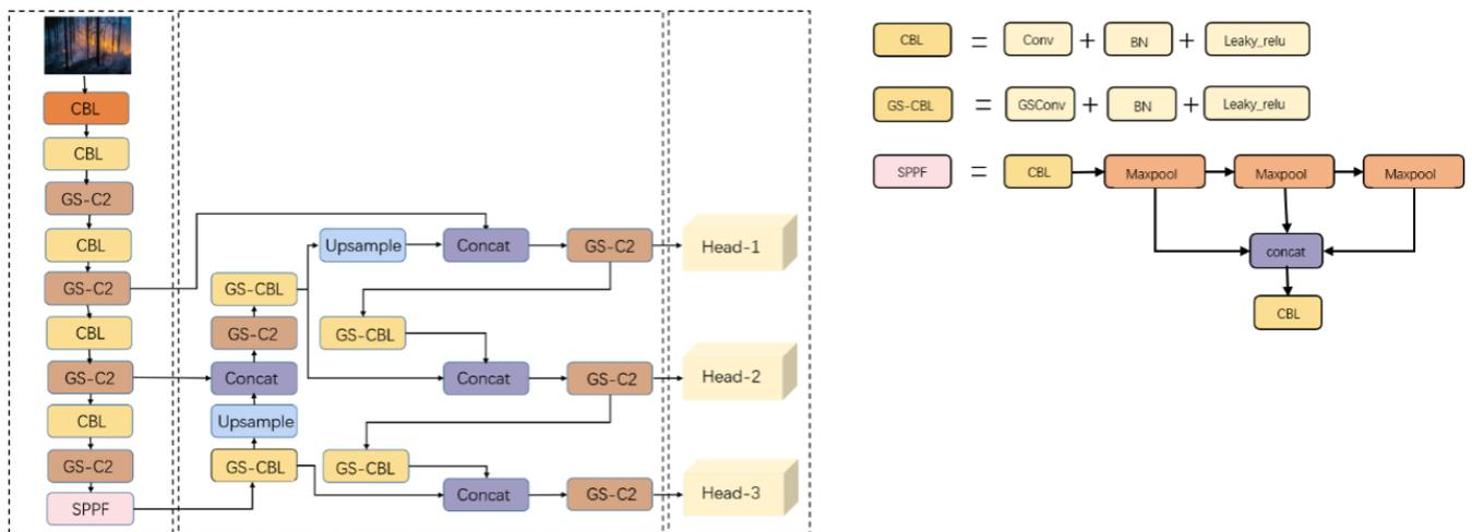
**Figure 8.** The overall architecture of the GS-YOLOv5 model, as well as the structural diagrams of the “CBL”, “GS-CBL”, and “SPPF” modules in the model.
