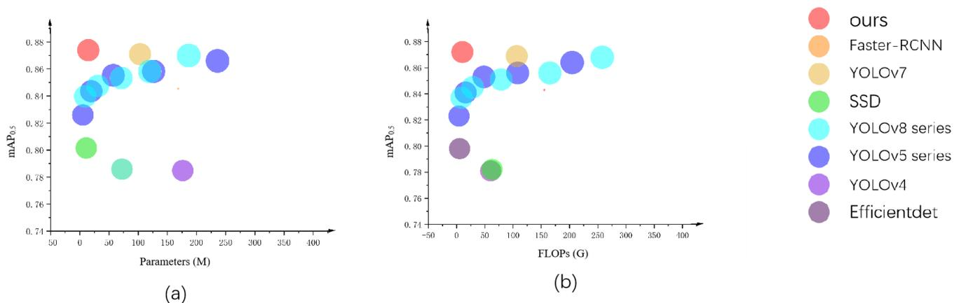
**Figure 9.** (a) Scatter plots of parameter numbers and  $mAP_{0.5}$  of the mainstream one-stage and two-stage detectors and GS-YOLOv5s; (b) scatter plots of FLOPs and  $mAP_{0.5}$  of mainstream one-stage and two-stage detectors and GS-YOLOv5s.
