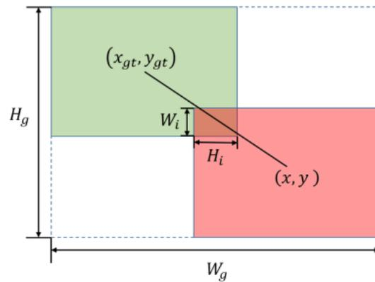
**Figure 5.** Map of the degree of overlap between the ground truth box (green) and the predicted box (red), where the blue dashed box represents the minimum closed box.
