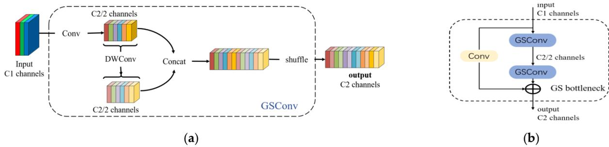
Figure 3. (a) GSCConv module. (b) GS bottleneck module.
