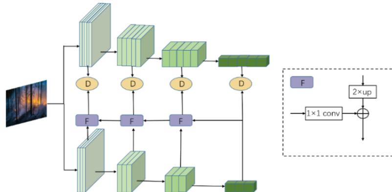
**Figure 7.** Structure diagram of the improved feature knowledge distillation network, where F is the feature fusion module.
