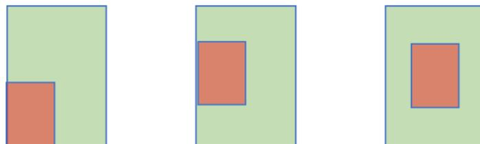
**Figure 6.** The performance of GIoU when the prediction box is completely contained within the target box; the red box represents the prediction box, and the green box represents the real box.
