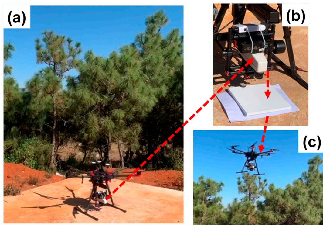
Figure 3. UAV hyperspectral imagery collection; (a) UAV on the ground; (b) Radiometric calibration; (c) The UAV in operation.
