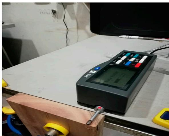
**Figure 4.** Surface roughness tester.
