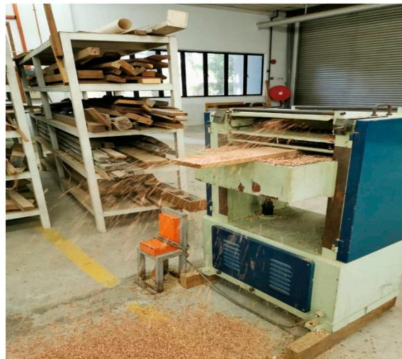
**Figure 2.** Thickness planer machine used for planing testing.
