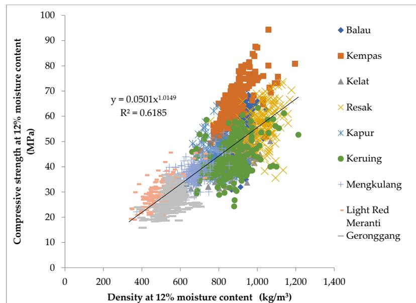
**Figure 6.** Relationship between compressive strength parallel to the grain and density for selected Malaysian tropical hardwood timbers.
