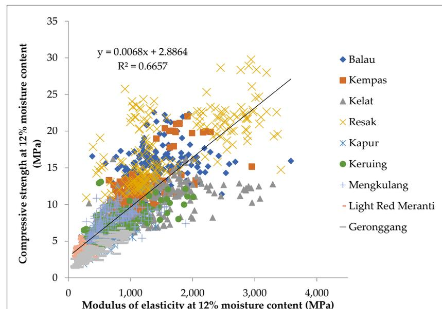
**Figure 5.** Relationship between compressive strength perpendicular to the grain and the modulus of elasticity for selected Malaysian tropical hardwood timber.
