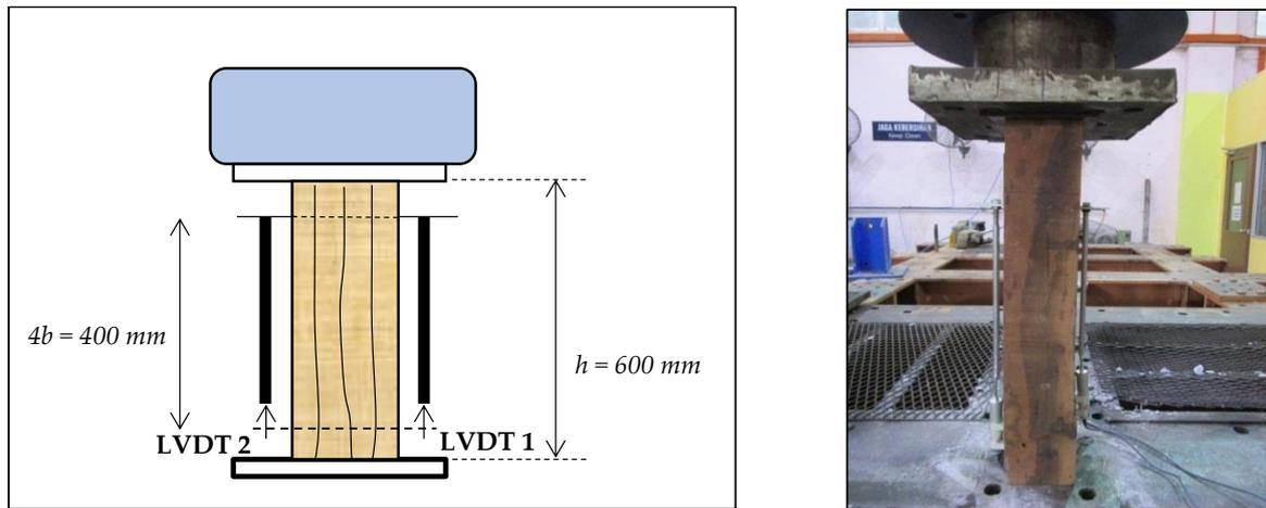
**Figure 2.** Test setup for determining compressive strength properties parallel to the grain.
