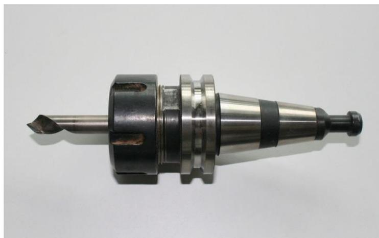
**Figure 1.** General view of the drill bit (shank part diameter—10 mm; shank length—27 mm; total length—70 mm; number of teeth—1) with a tool holder (ISO 30, ER 32).
