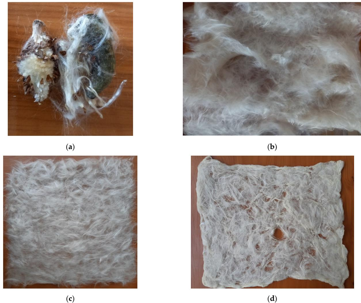
**Figure 2.** *Calotropis procera* fibres: (a) mature fruits; (b) extracted fibres arranged to form a thin sheet for composite layer; (c) untreated *Calotropis* sheet; (d) treated *Calotropis* sheet.
