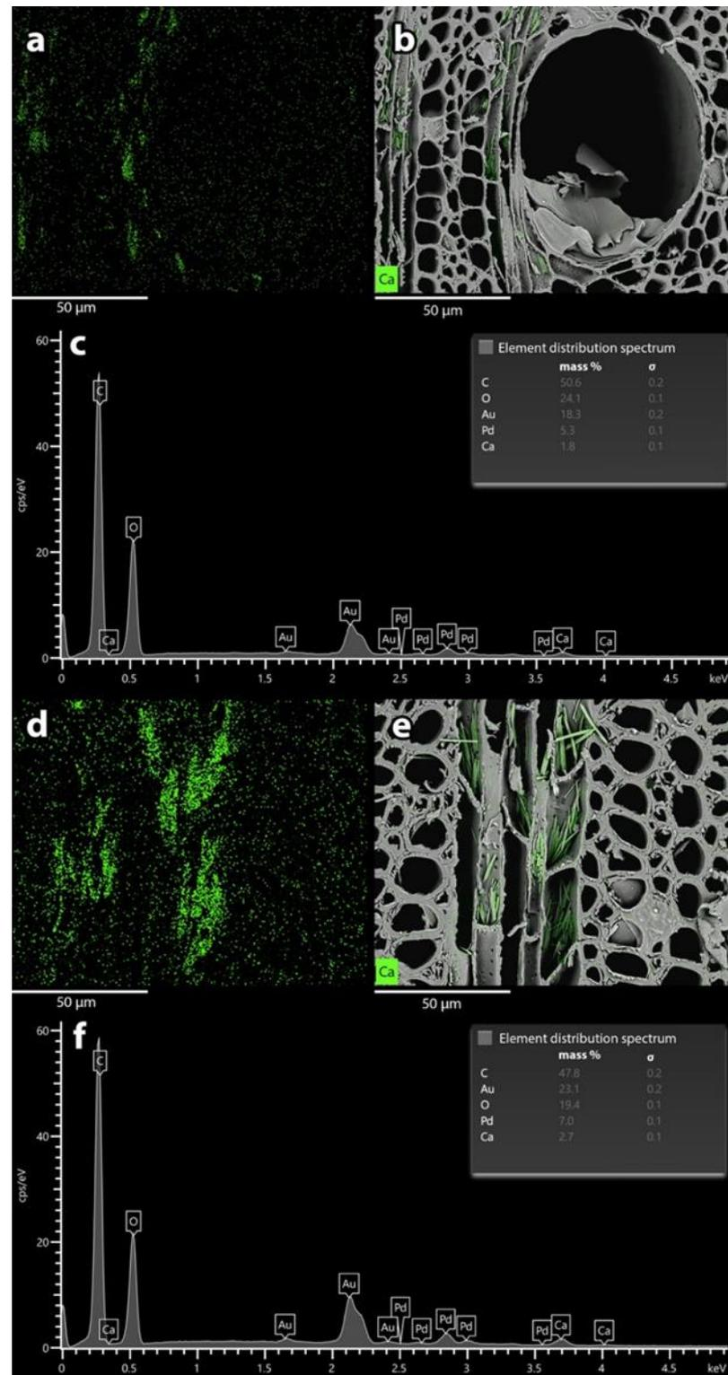
**Figure 4.** Needle-like crystalline structures found in the ray parenchyma cells of gmelina wood (a–d), present in large proportions and identified as calcium oxalate in the EDS spectrum (e,f).
