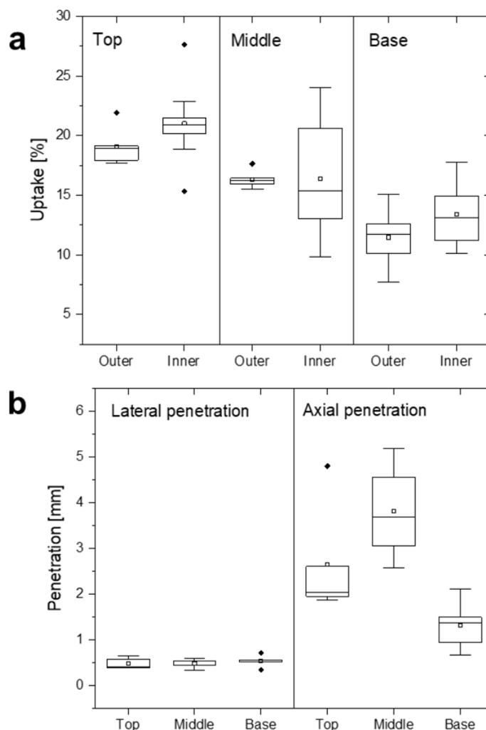
**Figure 2.** (a,b) Solution uptake and penetration depth of colored liquid in *Gmelina arborea* wood. The interpretation of the box plot is as follows: the centre line = the median, open square = the mean, box length = 25th to 75th percentile, whiskers 5th to 95th percentile, the black rhombus are the outliers.
