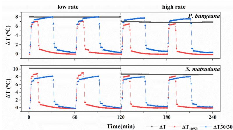
**Figure 3.** Temperature difference changes within hours of low (left side of dotted line) and high (right side of dotted line) sap flow rates under continuous heating ( $\Delta T$ , black), 10 min heating and 50 min cooling ( $\Delta T_{10/50}$ , red), and 30 min heating and 30 min cooling ( $\Delta T_{30/30}$ , blue).
