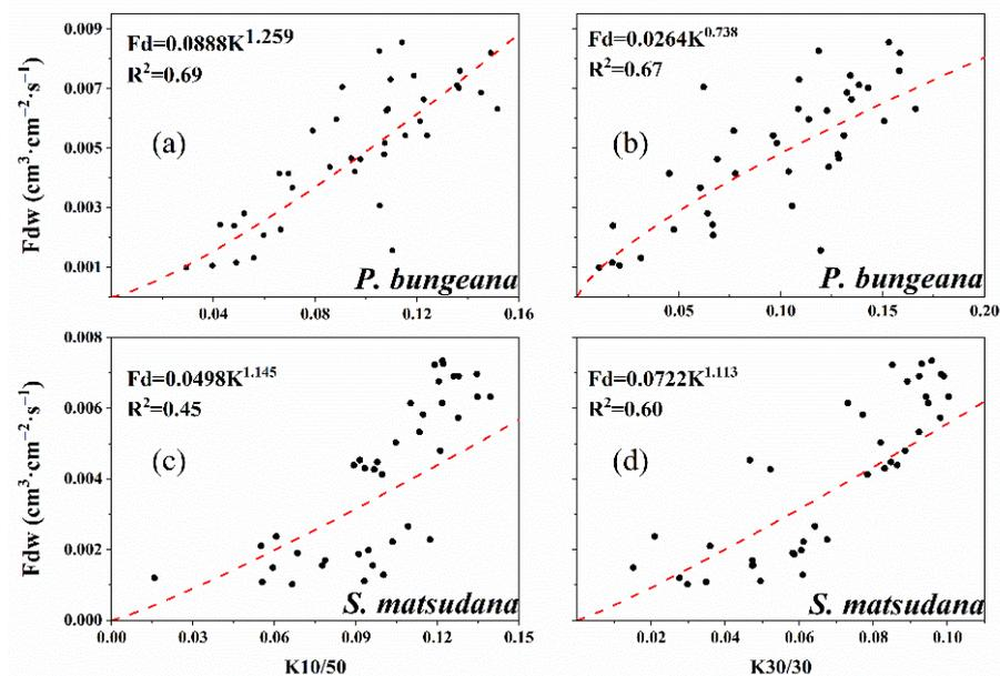
**Figure 4.** Relationship between  $K_{10/50}$  ( $K$  for 10 min heating and 50 min cooling mode, (a) and (c)) and  $K_{30/30}$  ( $K$  for 30 min heating and 30 min cooling mode, (b) and (d)) with reference sap flow density ( $F_{dw}$ , measured by tree weighing).
