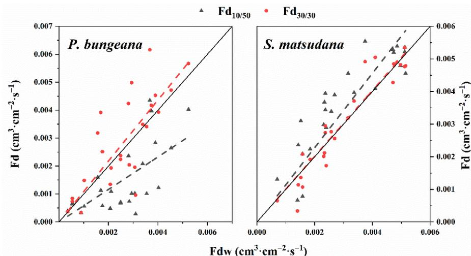
**Figure 5.** Verification of the accuracy of the calibration equations. The dashed black line represents the 10 min heating and 50 min cooling mode, the dashed red line represents the 30 min heating and 30 min cooling mode, and the solid black line is the 1:1 line.
