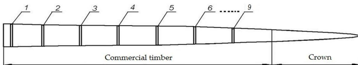
**Figure 1.** The scheme of cutting sections from the tree trunk: 9 cuts of wood cut from the trunk at 1 m intervals.
