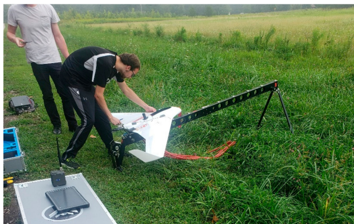
Figure 2. C-Astral Bramor Fixed-Wing Launching Mechanism.
