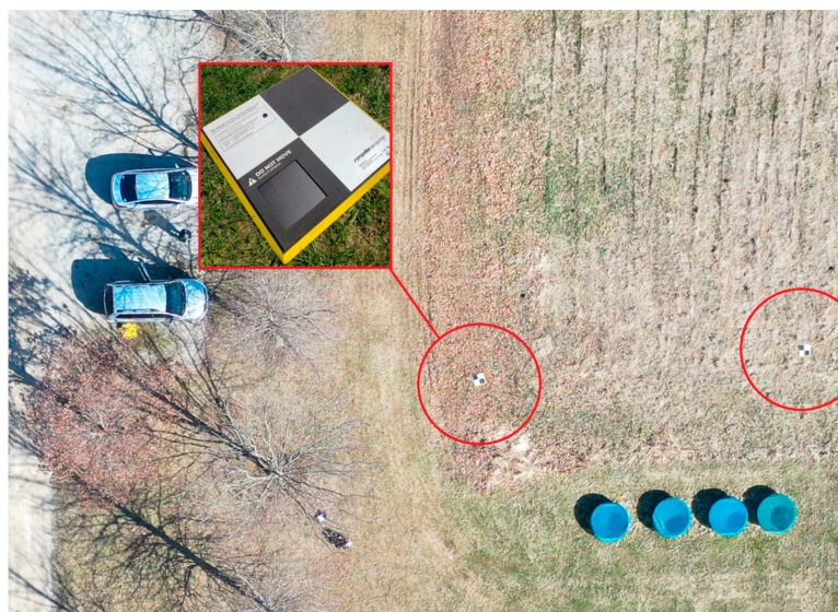
Figure 3. Aeropoint ground control point (GCP) markers (Outlined in Red) being utilized in a UAS data collection mission.
