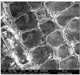
**Figure 8.** SEM images of the transverse faces of 30% FB01-treated sample 21. The left image is taken from the outer edge and the right image from the core of the sample. The spongy nature of the secondary walls appears to be reduced in both the surface and core, compared to the untreated reference shown in Figure 6. This may be attributed to the polymer within the cell walls.
