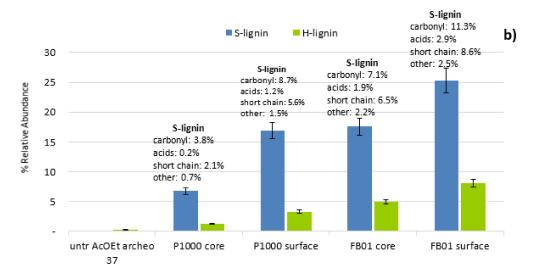
**Figure 10.** Distribution of (a) S-, G- and H-lignin units as percentages of lignin pyrolysis products identified in archaeological pine specimens treated with ethyl acetate (archeo AcOEt) and with P1000 and FB01 lignins, (b) S-lignin and H-lignin units as percentages of lignin pyrolysis products determined in P1000 and FB01 treated specimens are very low or absent in archaeological pine (products in red script in Table 2). Relative abundance is expressed as a percentage of total wood.
