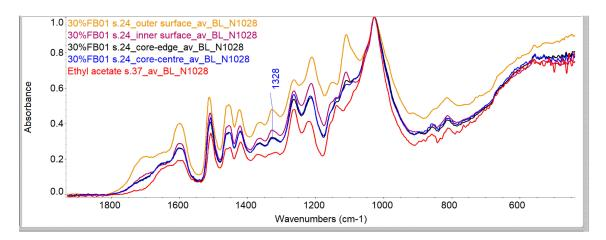
Figure 13. Comparing infrared spectra of 30% FB01-treated specimen 24 from different depths to assess penetration from outside to inner core by measuring band heights at  $1328 \, \mathrm{cm}^{-1}$ . The ethyl acetate-treated control (nr. 37) is shown in the red curve. The image shows 'outer surface' (orange), 'inner surface (purple), 'core edge' (black) and 'core centre' (blue). All spectra were baseline corrected and normalized to  $1028 \, \mathrm{cm}^{-1}$ .
