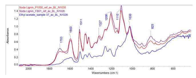
**Figure 11.** Comparing lignins to ethyl acetate-treated archaeological wood (nr. 37). Infrared spectra of lignin P1000 (red curve), FB01 (purple curve) and of wood (blue curve) were baseline corrected and normalized at  $1028 \text{ cm}^{-1}$ . The band height used to measure extent of penetration of lignins into the wood samples is shown at  $1327 \text{ cm}^{-1}$ .
