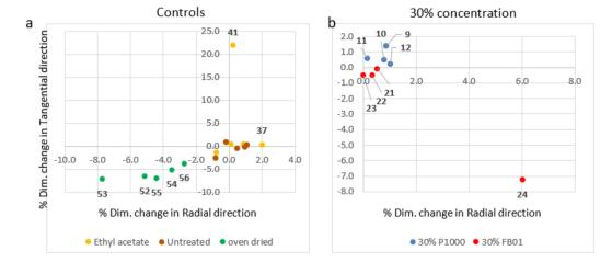
**Figure 5.** % Dimensional change plotted as % tangential change (y-axis) vs. % radial change (x-axis). (**a**) Controls, where only data points with largest changes are labelled; (**b**) 30% concentrations of P1000 and FB01 lignins. Data points are labelled with specimen number.
