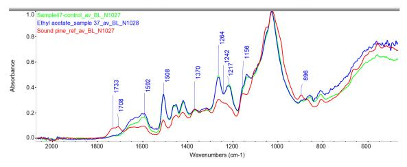
**Figure 3.** Infrared spectra of archaeological wood, untreated specimen nr. 47 (green curve), ethyl acetate-treated control nr. 37 (blue curve) and sound pine (red curve). Main differences are highlighted at indicated bands.
