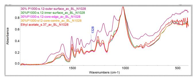
**Figure 12.** Comparing infrared spectra of 30% P1000-treated specimen 12 from different depths. Bands at  $1328 \text{ cm}^{-1}$  were measured. The ethyl acetate-treated control is shown in the red curve (nr. 37). The image shows 'outer surface' (purple), 'inner surface (green), 'core edge' (pink) and 'centre core' (orange). All spectra were baseline corrected and normalized to  $1028 \text{ cm}^{-1}$ .
