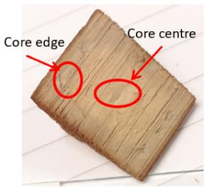
**Figure 1.** Areas sampled for infrared analyses: 'outer surface', 'inner surface', 'core edge' and 'core centre. For Py-GC/MS, only 'inner surface' and 'core centre' were analysed. These depths were used to evaluate penetration of the polymer.
