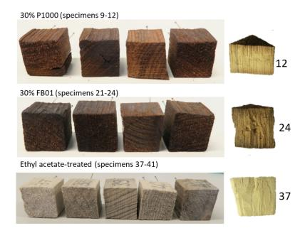
**Figure 4.** Specimens treatment with 30% lignins P1000, FB01 (w/v) and the control (ethyl acetate-immersed) after air-drying. Specimens 12, 24 and 37 are also shown after they were cut in half for sampling.
