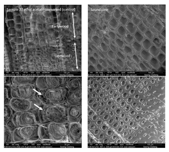
**Figure 6.** SEM images of the transverse faces of ethyl acetate-immersed sample 37 (control) on the left panel and of sound pine on the right panel. The upper right image shows the earlywood of sound pine, and the bottom right shows latewood cells of sound pine. The lower left image, which magnifies a region of latewood, shows the spongy nature of the secondary walls (arrows) in the archaeological sample.
