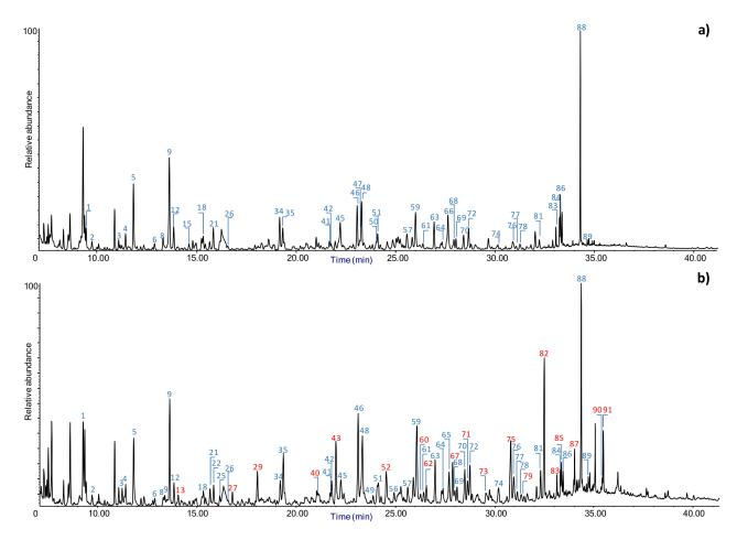
**Figure 9.** Chromatographic profiles obtained by Py(HMDS)-GC/MS (a) archaeological pine (specimen 47) and (b) archaeological pine treated with FB01 (specimen 22). Lignin pyrolysis products, which were very low or absent in archaeological pine, were used to evaluate lignin penetration in test specimens. These are labelled in red script. Peak numbers refer to Table 2.
