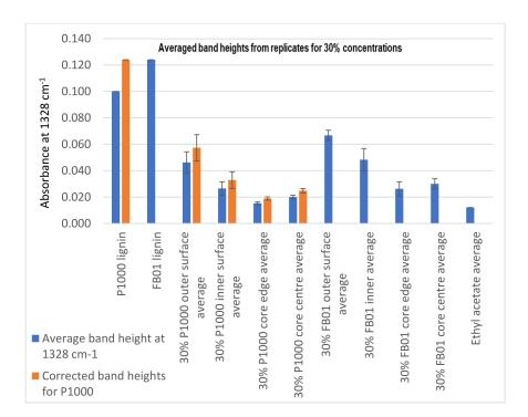
**Figure 14.** Comparing band heights measured from infrared spectra for 30% concentrations. The band heights from each depth were averaged for each treatment group (4 replicates): 'outer surface', 'inner surface, 'core edge' and 'core centre'.
