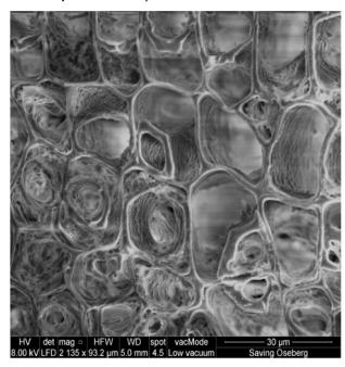
**Figure 7.** SEM images of the transverse faces of 30% P1000-treated sample 9. The left image is taken from the outer edge and the right image from the core of the sample. The spongy nature of the secondary walls appears to be reduced in the surface and only slightly reduced in the core, compared to the untreated reference shown in Figure 6. This may be attributed to the polymer within the cell walls in the surface.
