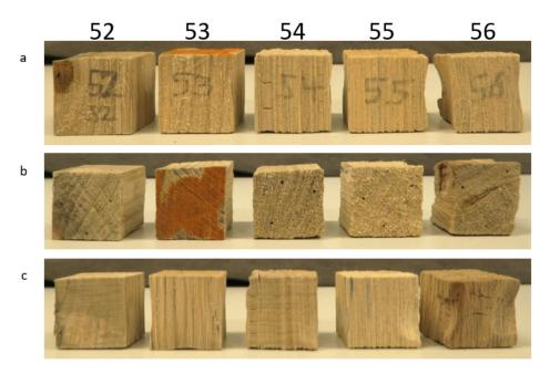
**Figure 2.** Samples used for wood characterization after oven-drying. Images show variability in samples: (a) nr. 52 has a knot (dark spot on upper left corner), 54 shows cross-grained cracking after freeze-drying or oven-drying. (b) nr. 53 has orange staining on it transverse section, possibly iron compounds. Additionally, note that the annual rings are not aligned with sample sides. (c) nr. 56 shows cross-grained cracking after freeze- or oven-drying.
