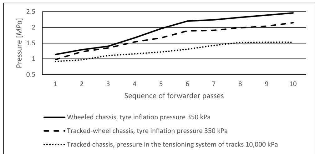
**Figure 9.** Soil profile compaction at a depth of 15 cm during ten passes of three chassis variants of the loaded forwarder.
