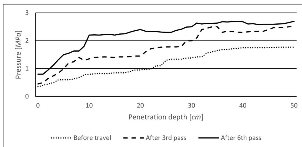
**Figure 8.** Soil profile compaction before travel, and after the third and sixth pass of the loaded wheeled forwarder.
