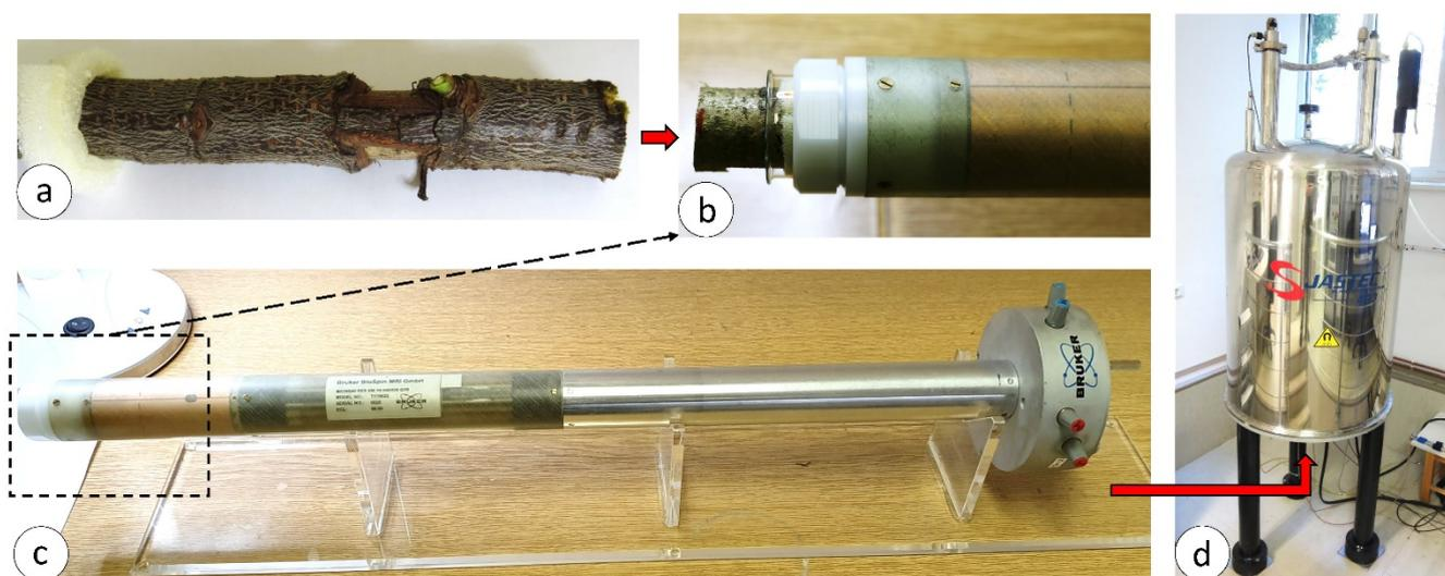
**Figure 1.** (a) Sample PrLa\_76 (*Prunus laurocerasus*); (b,c) 30 mm diameter RF coil (Bruker, Ettlingen, Germany) and (d) MRI spectrometer with a superconducting 9.4 T magnet (Jastec 400, Kobe, Japan).
