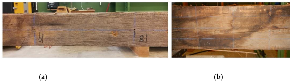
Figure 3. The ground-penetrating radar (GPR) scan lines of the timbers. (a) The middle scan line on B or D side; (b) Three scan lines on C or E side.
