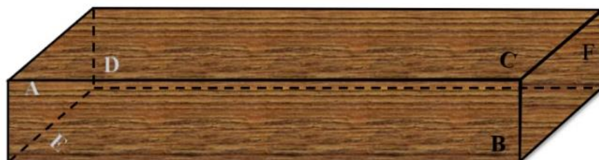
Figure 2. The three-dimensional model of the timbers. A and F are the left and right sides, E and C represent the bottom and top sides with 381 mm width, B and D denote the front and back sides with 101.6 mm thickness.
