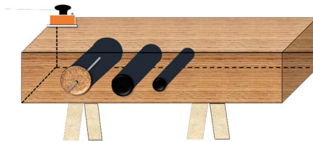
Figure 9. GPR scanning after inserting core-samples into the timber section.
