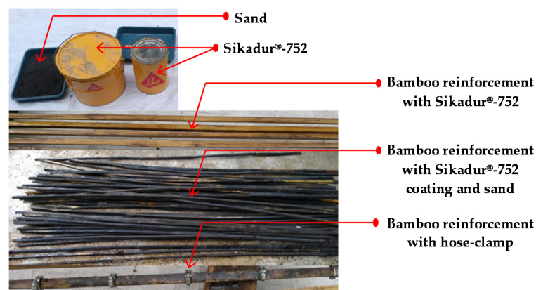
Figure 1. The materials and treatments of bamboo reinforcement.
