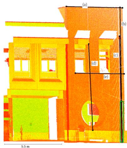
**Figure 7.** Laser scanning 3D point cloud of the test area including the segments (a–e). Green portion: The reference scale bar used to constrain the photogrammetric model; black lines: Distances used for validation.
