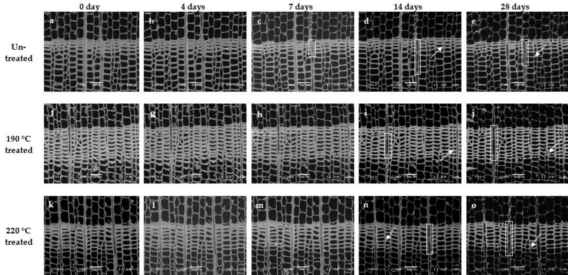
Figure 3. Scanning electron micrographs of cross sections of untreated and heat-treated wood before and after natural weathering.
