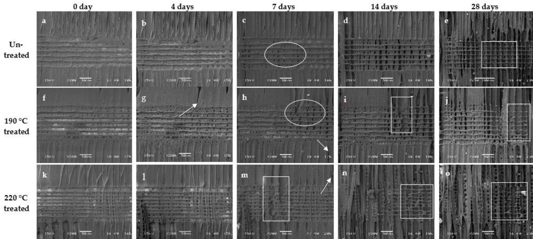
**Figure 4.** Scanning electron micrographs of radial sections of untreated and heat-treated wood before and after natural weathering.
