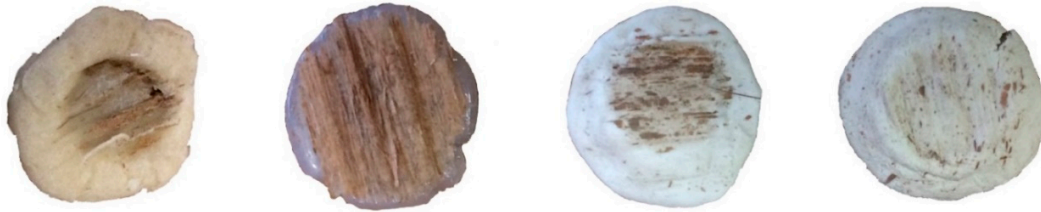
Figure 3. From left to right: Wheat flour, ethylene-vinyl acetate copolymer (EVA), calcium carbonate, aluminosilicate.
