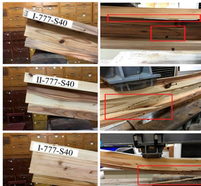
**Figure 6.** Failure usually resulting from the bottom flange at the position directly below the loading position.
