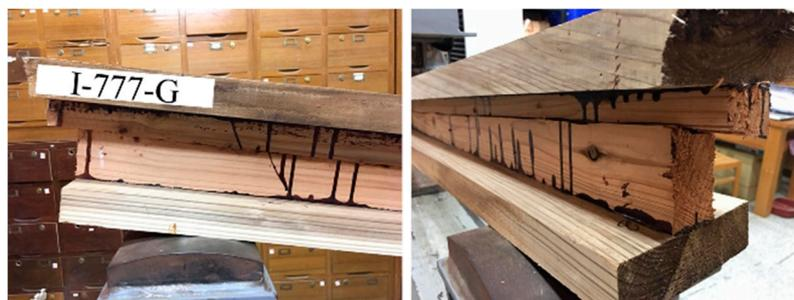
**Figure 8.** Horizontal shear failure at the web of the built-up I-beams.
