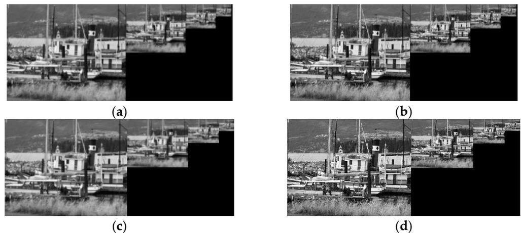
**Figure 3.** Comparative effects of different methods for constructing scale spaces. (a) Gaussian filtered average downsampling image. (b) Gaussian filtered maximum downsampling image. (c) Nonlinear average downsampling image. (d) Nonlinear maximum downsampling image.
