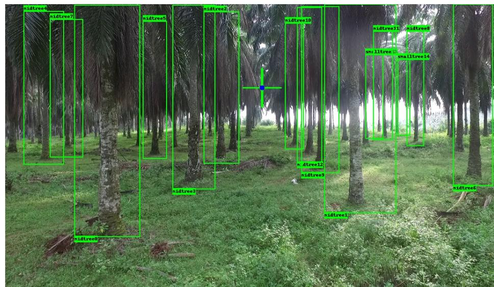
**Figure 1.** Sample frame from the drone vision system depicting the detected objects and the guided localization point in the frame.
