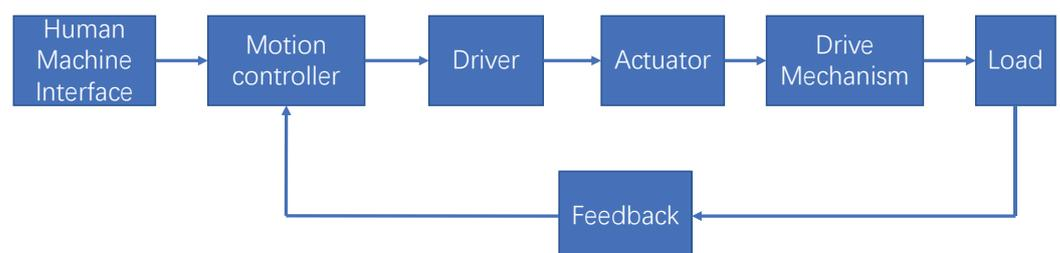
**Figure 1.** Structure diagram of servo motor control system.
