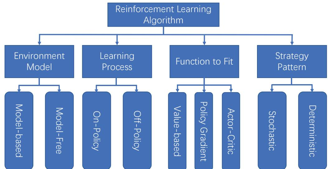
**Figure 2.** Classification of reinforcement learning algorithms.
