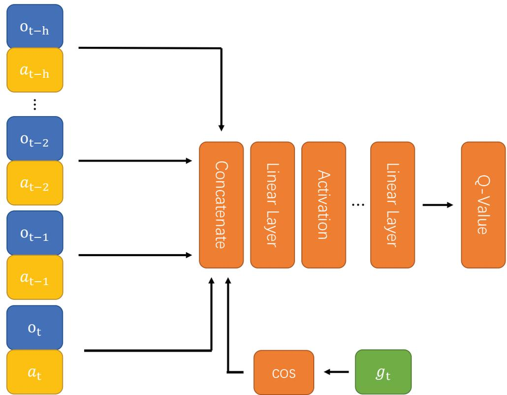
Figure 4. The structure of the value network.
