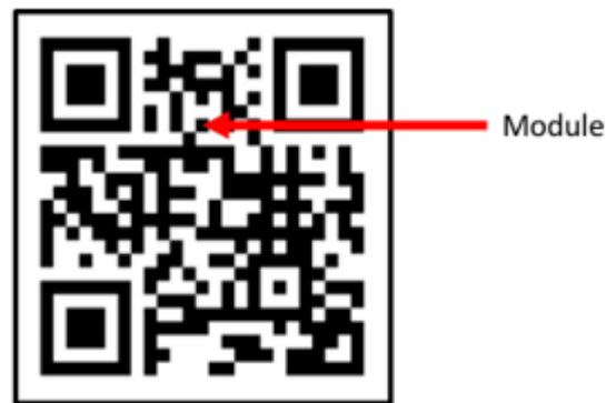
Figure 1. QR code basic unit diagram.
