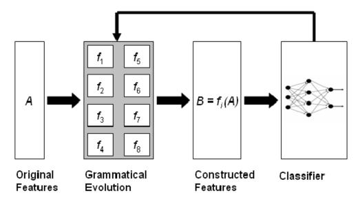
Figure 1. Schematic representation of the feature construction technique.
