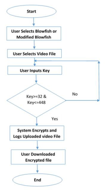
Figure 2. System Flowchart for the proposed modified algorithm.
