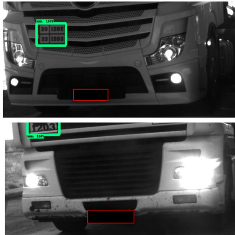
**Figure 6.** Examples of ADR-Det algorithm successful ADR sign detection (green image box), using an evaluation dataset of 500 ADR images.
