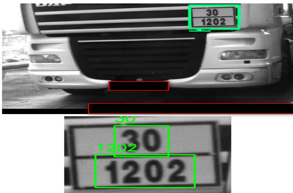
**Figure 4.** HMRT-EF OCR process with its OCR preview capabilities enabled displaying the detected Regions of Interest.
