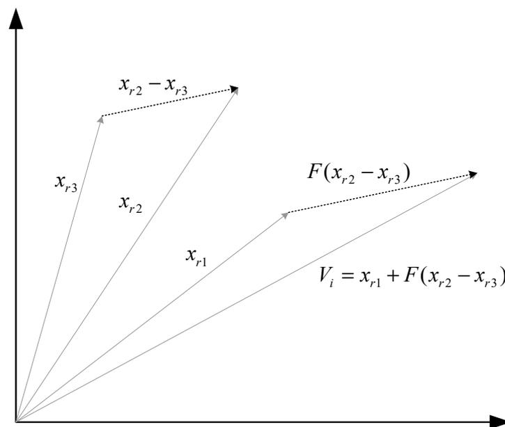
**Figure 2.** Basic idea of differential evolution algorithm.
