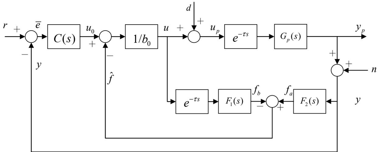
Figure 7. Control structure.
