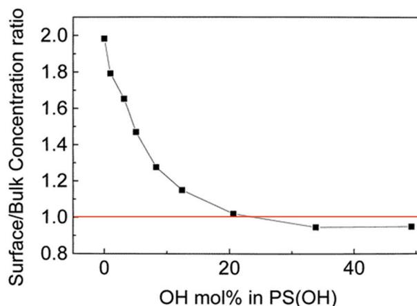
**Figure 12.** Ratio of PS(OH) concentration at the surface to PS(OH) concentration in the bulk in PS(OH)/PVPy blends vs. the HFMS content in PS(OH) [20].
