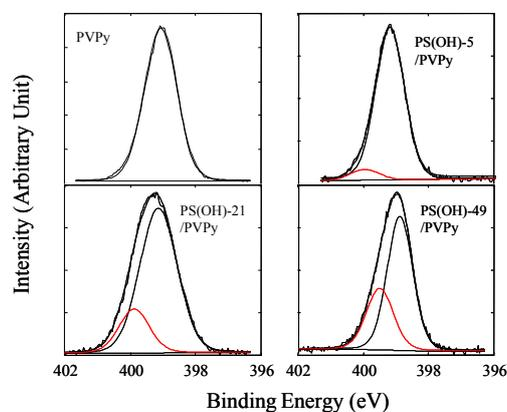
**Figure 10.** XPS N1s core-level spectra of pure PVPy, the PS(OH)-5/PVPy blend, and the PS(OH)-21/PVPy and PS(OH)-49/PVPy complexes [21].
