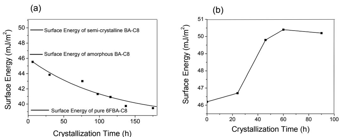
**Figure 4.** (a) Plot of the surface energy of the BA-C8/6FBA-C8 (80/20) blend as a function of crystallization time (b) plot of the surface energy of BA-C8 as a function of crystallization time [42].
