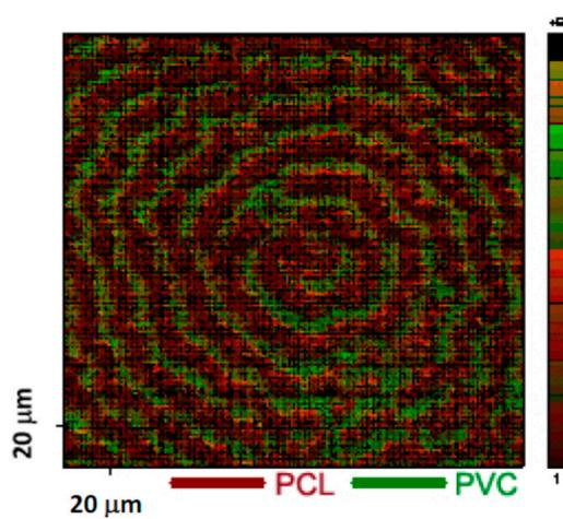
Figure 3. Ion map of the blend of PCL and PVC grown at 45 °C [41].
