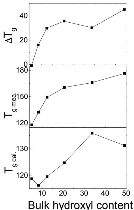
**Figure 9.** Calculated and measured  $T_g$ s for the PS(OH)/PVPy blends or complexes as a function of the hydroxyl content in PS(OH) [21].
