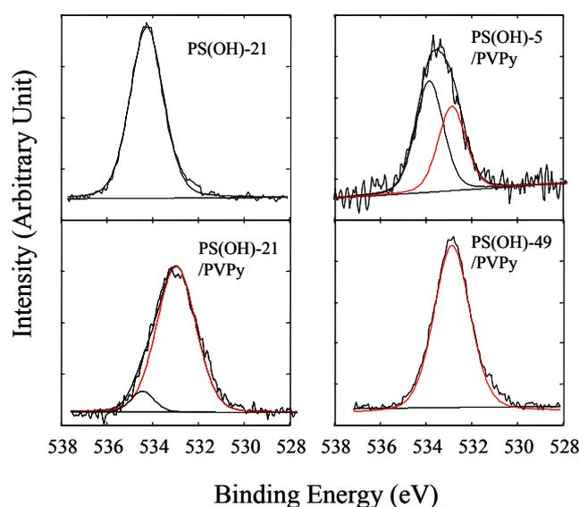
**Figure 11.** XPS O1s core-level spectra of pure PS(OH)-21, the PS(OH)-5/PVPy blend, and the PS(OH)-21/PVPy and PS(OH)-49/PVPy complexes [21].
