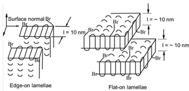
Figure 2. Schematic showing edge-on and flat-on lamellae [45].
