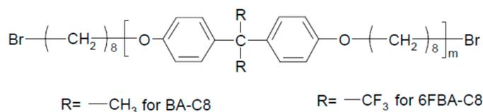
**Scheme 2.** Structure of BA-C8 and 6FBA-C8 [47].
