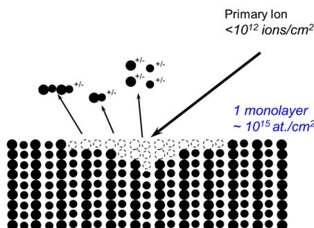
**Scheme 1.** Schematic of a static SIMS process.
