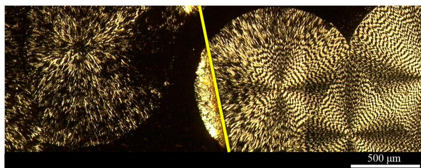
**Figure 7.** A polarizing optical micrograph of spherulites that formed in a 3  $\mu$ m thick film of a PLLA/PEO (50/50) blend crystallized in air at 125 °C for five hours on a glass slide. The right half of the sample was placed under a glass coverslip [42].
