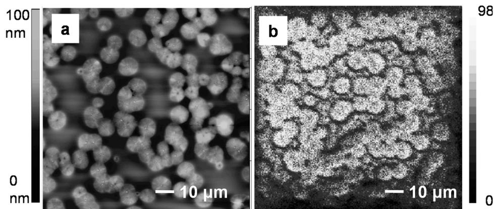
**Figure 5.** AFM height image (a) and the corresponding ToF-SIMS  $F^-$  image (b) for the BA-C8/6FBA-C8 (80/20) blend 68 h after it was prepared [42].
