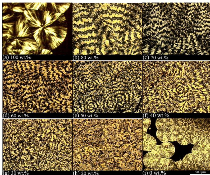
**Figure 6.** Polarized optical micrographs of 3- $\mu$ m-thick films: (a) poly(L-lactic acid) (PLLA) and (b–h) PLLA/poly(ethylene oxide) (PEO) blend films sandwiched between two glass slides after annealing in air at 125 °C for five hours for different PLLA weight concentrations; (i) a PEO film sandwiched between two glass slides after annealing in air at 50 °C for two minutes [42].
