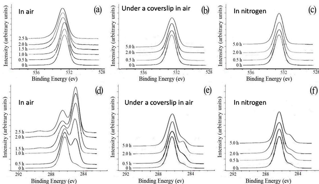
**Figure 8.** O1s spectra (a–c) and C1s spectra (d–f) of the original PEO films and PEO films annealed at 125 °C for up to 5 h: (a,d) without a coverslip in air; (b,e) with a coverslip in air; (c,f) without a coverslip in nitrogen [42].
